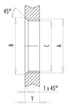
Installation direction: o-ring sits on chamfer.
